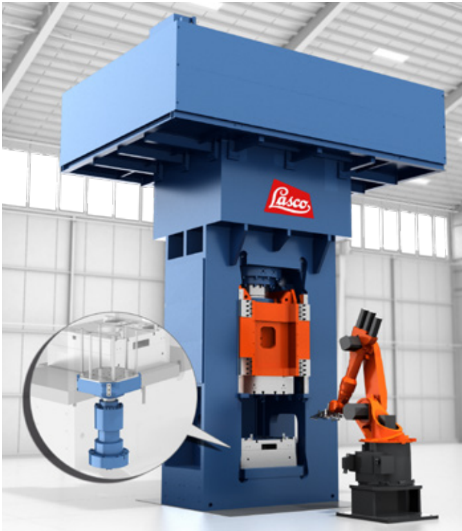
LASCO blanking press with schematic representation of the drawing cushion
