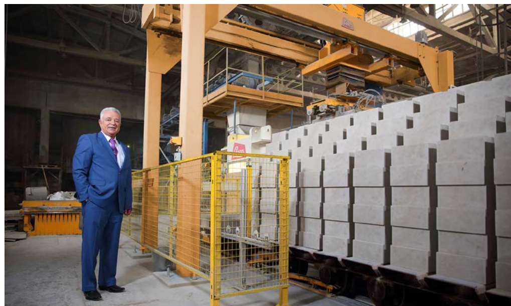
Vladimir Barankov in the modern production hall with sand-lime green blocks stacked appropriately for the autoclave. The enterprise ranks among the top 50 of the building and building material sector in the Russian Federation.
