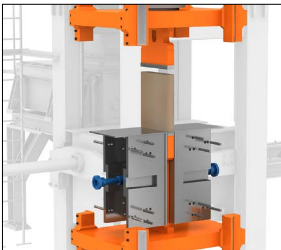
Pressing and ejection of the format 115 mm wall thickness
