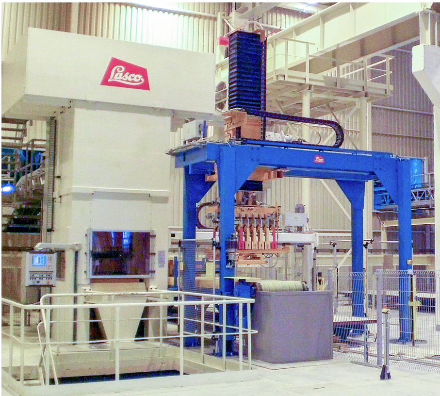
At AB Silikatas Akcine Bendrove in Vilnius, a modern KSP 801 from LASCO replaces an old mechanical press.
