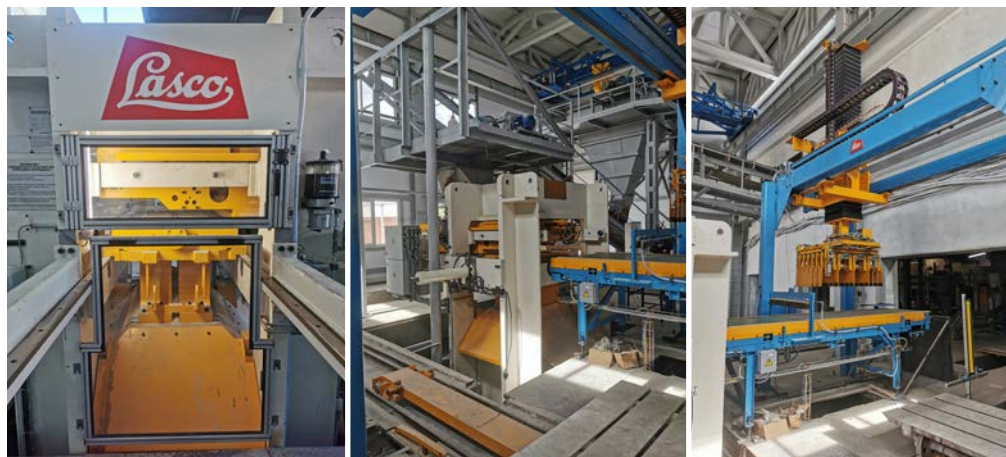
Pictures taken in the production hall of TOO “Silikat” Semej during the assembly of the new sand-lime block press KSE 401 B from LASCO.
