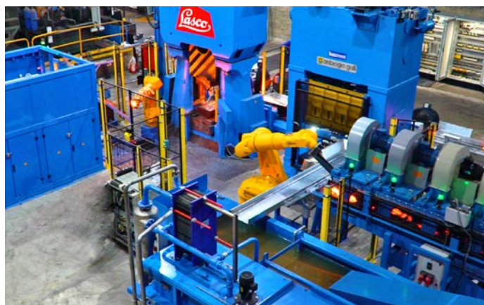
Semi-automatic forging line with LASCO HO-U 500, step feeder, heating system and robots.
