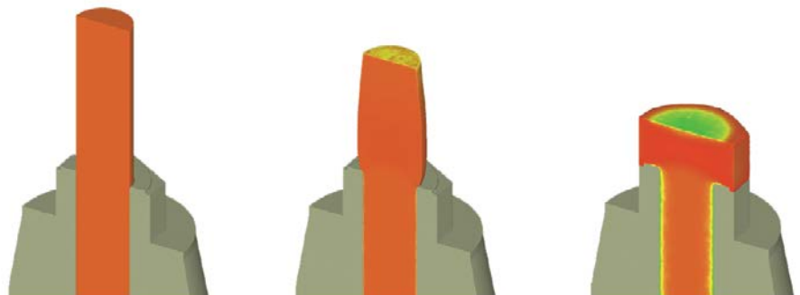
Picture 2: Simulation representation of a coning and finish-forming operation
