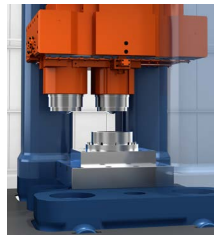
Picture 3: Shifting slide with two upper dies
