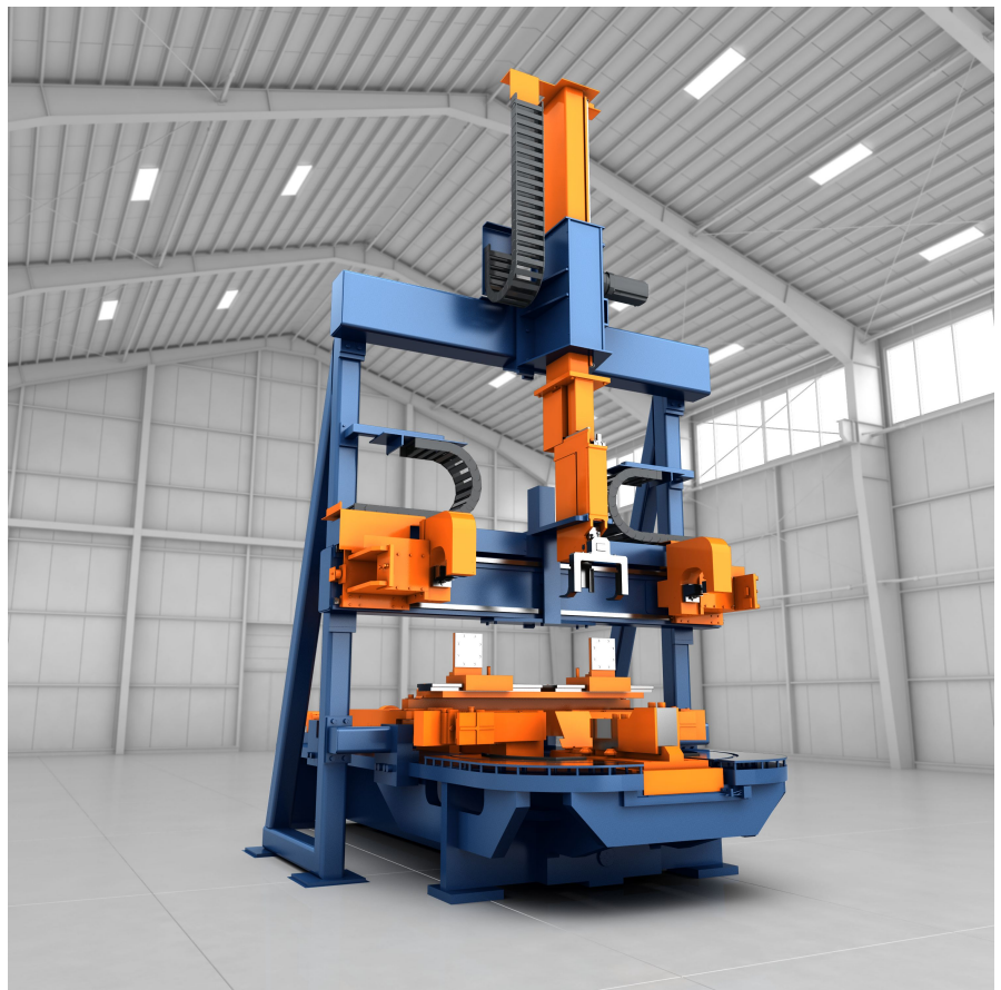
Picture 5: LASCO system for bending, calibrating and coining
