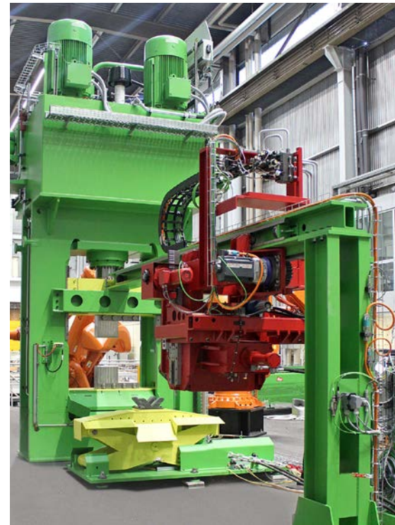
With the automatic LASCO stretching system AR 250/250, GGF has now modernized the first of its five forging lines. The picture shows the system during assembly in Coburg.
