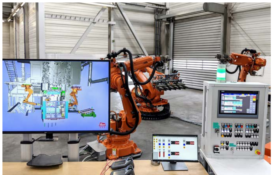
While production continues on the real forging system, the robots are programmed in active interaction with the digital model.
