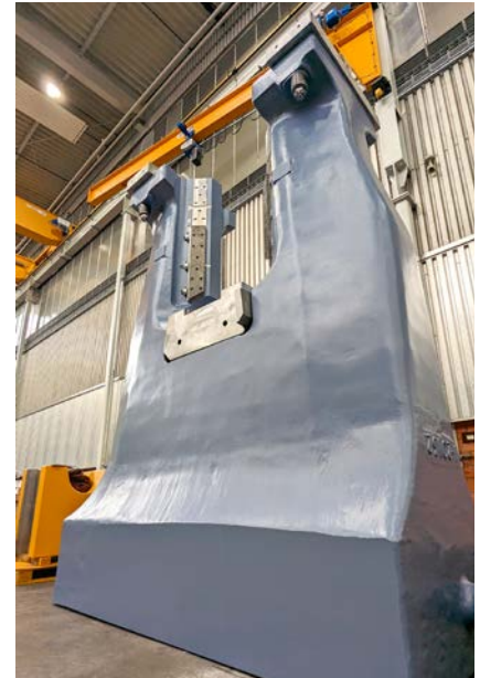
The massive U-frame of the new forming unit alone, weighing approx. 58 t, is an imposing sight.
