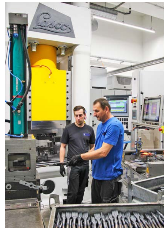
The DreBo tool factory in Althausen has been using a state-of-the-art LASCO screw press for the production of high-quality drilling tools for several months.
